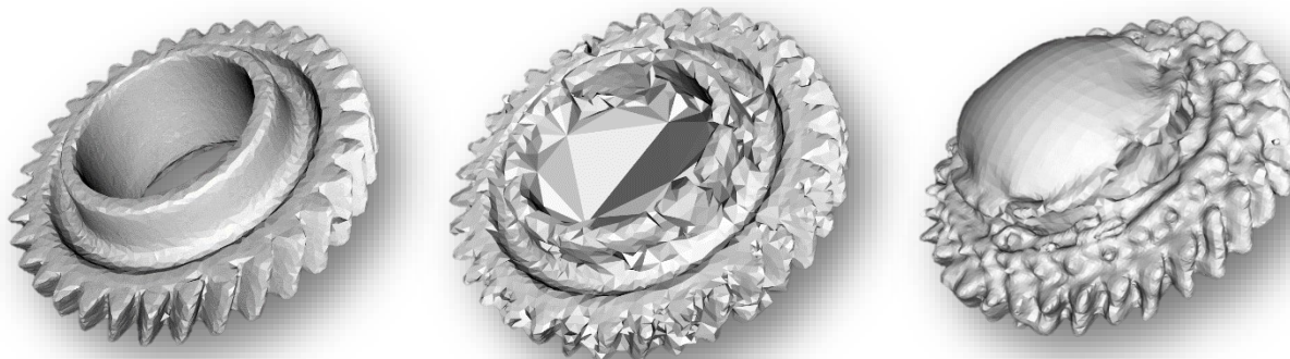
Figure 8. sGNG (left) reconstructed the center hole and the teeth of the gear very well, GCS (middle) showed worse results in reconstruction of the hole due to the specifics of the algorithm. PCL Poisson reconstruction (right) is significantly worse.
