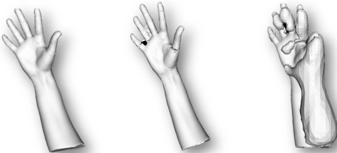
Figure 14. sGNG (left) reconstructed smooth arm surface, GCS (middle) produced arm with a few cuts and “webbed fingers”. PCL Poisson algorithm (right) reconstructed arm with an unexpected part.
